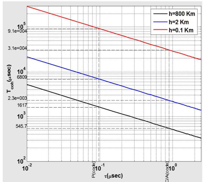
Fig.4: coherent time  $T_{coh}$  versus versus chip period  $\tau$
