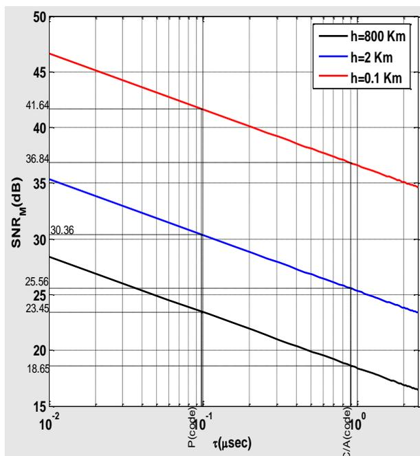
Fig.5:  $SNR_M$  versus versus chip period  $\tau$
