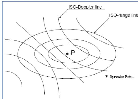
**Fig.2. The footprint area of GPS scattering signal on the earth's surface**
