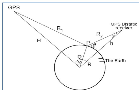
Fig.1. Geometry of GPS bistatic system
