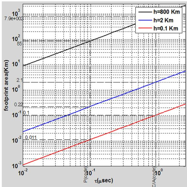
Fig.3: Footprint area versus versus chip period  $\tau$
