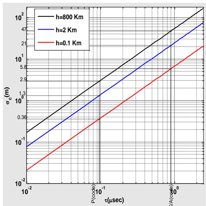
Fig.6: range rms error  $\sigma_c$  versus versus chip period  $\tau$
